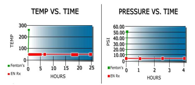
The success of in-situ chemical oxidation technology is dependent on effectively delivering chemical oxidants to the contaminant impacted groundwater. The delayed calorie release allows EN Rx Reagent<sup>™</sup> to be applied at very low pressure. The goal is to elevate groundwater to cover the vadose zone and use head pressure to naturally migrate reagent through groundwater void space.
